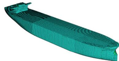
MAESTRO also provides fine meshing capabilities which allow the global model to be automatically refined while maintaining the original scantling properties and loads. The fine mesh model(s) can be analyzed as a separate model or integrated into the global model. Either option automatically applies the appropriate boundary conditions to impose the global loads onto the fine mesh model(s).
