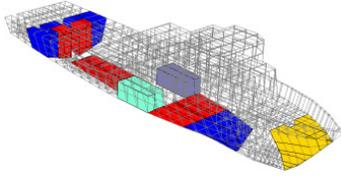
and permeability and automatically manages the element pressure side, even for elements shared between tank boundaries. Tank loads can be varied between load cases allowing the user to create multiple conditions within a single model. For each load case, a tank table is available summarizing the tank volumes, loads, and centers of gravity.
