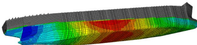
design waves) are internally computed and selected for assessment of extreme global loads. The user has a variety of options to add still water loads to the wave-induced loads and to re-balance these components.
