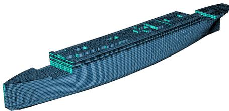
found within portions of a ship (e.g., plating thickness or frame size throughout a cargo hold, etc.). Each module has its own local coordinate system, and can be copied, rotated or transformed. This paradigm not only supports the rapid *creation* of the finite element model but also the *modification* of the finite element model, which is routinely required
