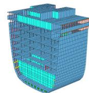
during the design process. Hull girder properties such as inertias, cross-sectional area, neutral axis, and section modulus can be plotted and queried for any section cut within the model.
