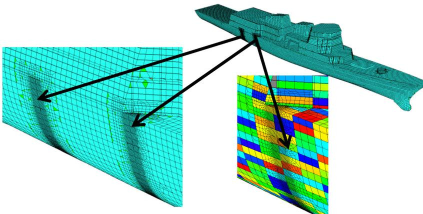
capabilities available to the ship structural engineer, and results in a comprehensive level of information that identifies structural problems associated with events such as buckling. These structural failure evaluations are used by the structural engineer to assess the adequacy or degree of conservatism
