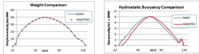
Fig.2 Weight and Buoyancy Distribution Comparison
