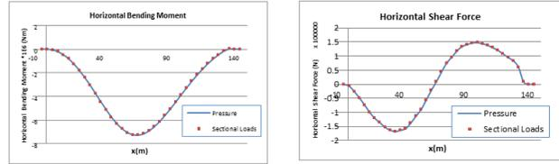
**Fig. 14 Horizontal Bending Moment and shear force**
