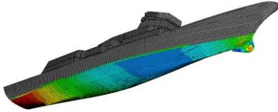
**Fig. 11 Hydrodynamic Pressure Distribution**
