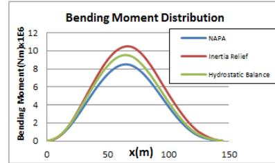
Fig. 8 Comparison of bending moment distribution
