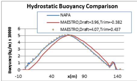
Fig.5 Buoyancy distribution comparison with MAESTRO auto-balancing
