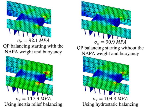
**Fig. 9 Comparison of the main deck longitudinal stress distribution**
