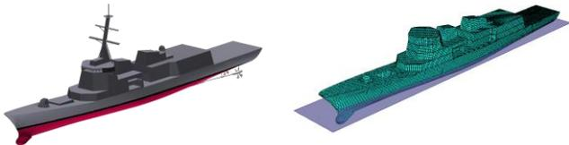
Fig.1 Finite element model generated from the NAPA molded form model
