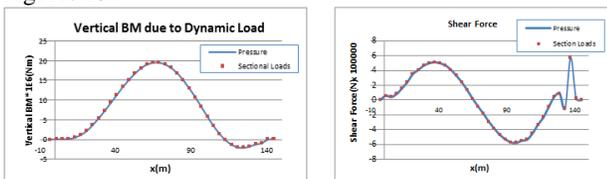
**Fig. 12 Vertical bending moment and shear force**
